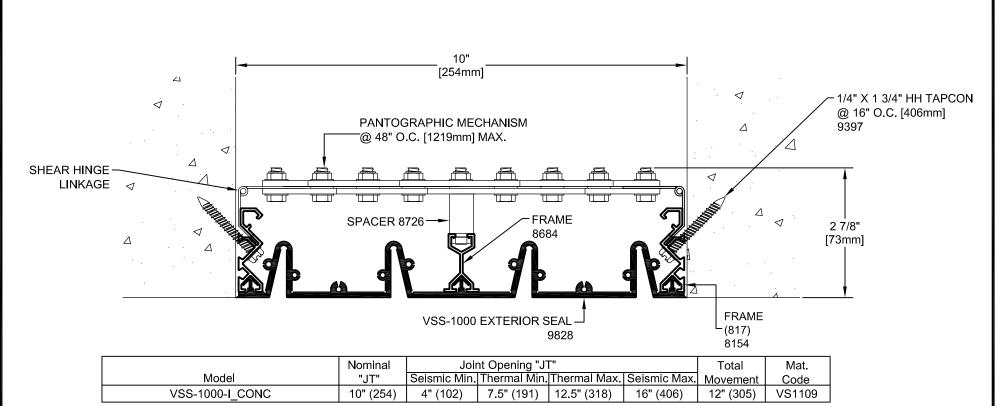
NOTE THAT EXTERIOR SEAL DISENGAGES AT 15". ( ) IN MOVEMENT TABLE DENOTES mm IN METRIC.
